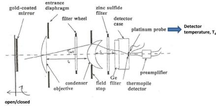
**Radiance measured in band i:**  $L_i = B_i(T_d) + \Delta L_i$
