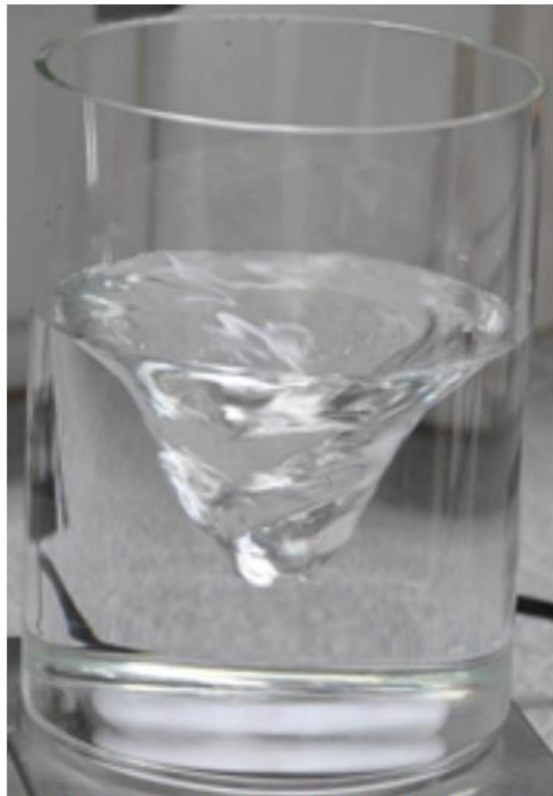
Figure 4: Cone-shaped vortex in water as a simple calibrator.
