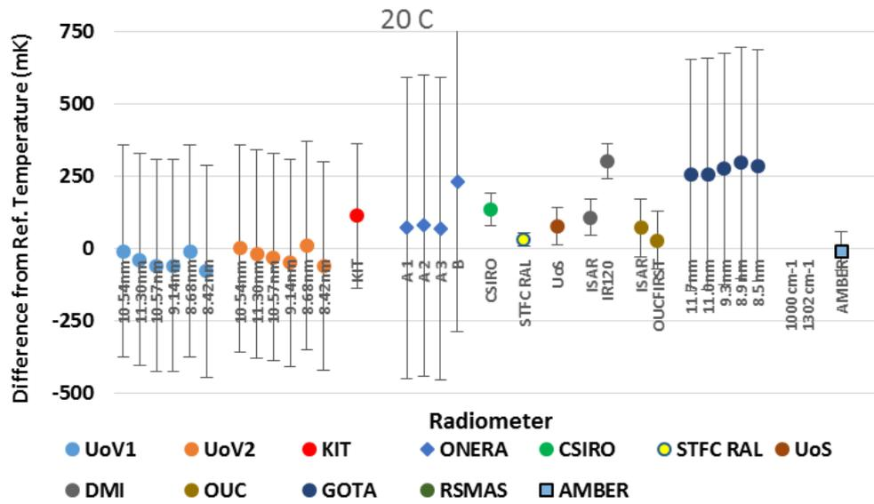
**Figure 7:** Plot of the mean of the differences of the radiometer readings from the temperature of the NPL reference blackbody, maintained at a nominal temperature of 20 °C.
