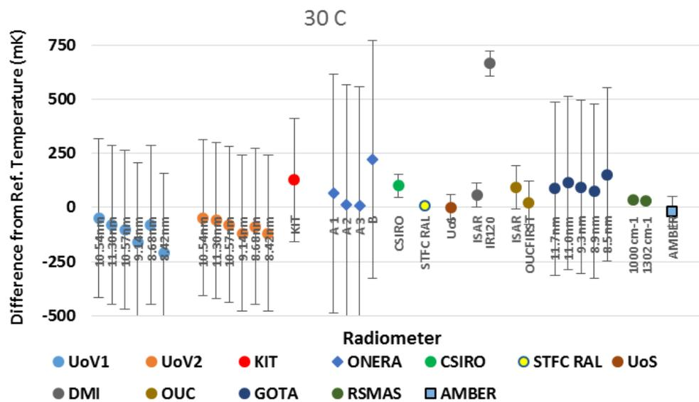
**Figure 8:** Plot of the mean of the differences of the radiometer readings from the temperature of the NPL reference blackbody, maintained at a nominal temperature of 30 °C.
