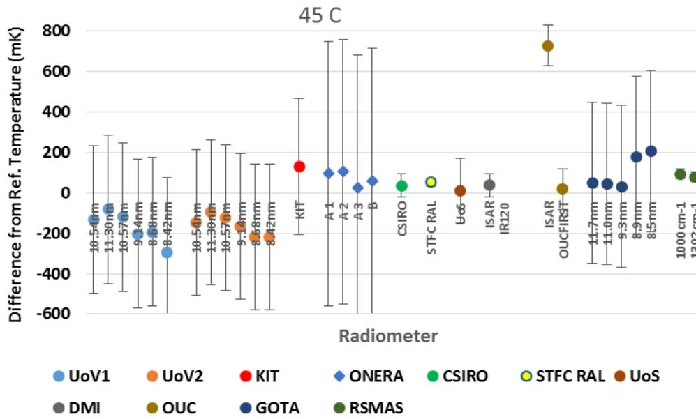
**Figure 9:** Plot of the mean of the differences of the radiometer readings from the temperature of the NPL reference blackbody, maintained at a nominal temperature of 45 °C.
