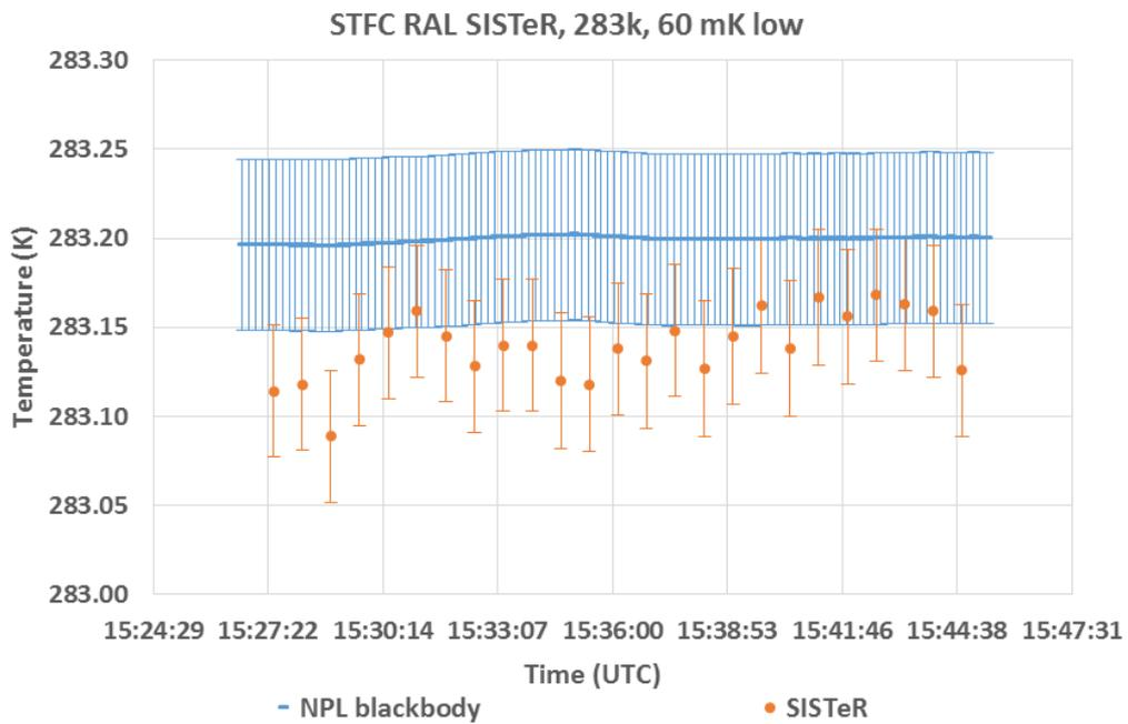
**Figure 2:** Measurements of the STFC RAL SISTeR radiometer viewing the NPL reference blackbody maintained at approximately 10 °C (in orange) and the corresponding measurements made by NPL of the blackbody temperature (in blue).
