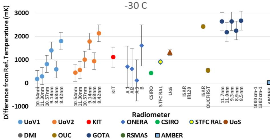
Figure 3: Plot of the mean of the differences of the radiometer readings from the temperature of the NPL reference blackbody, maintained at a nominal temperature of -30 °C.
