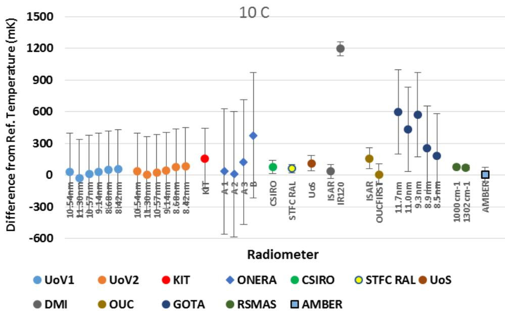
Figure 6: Plot of the mean of the differences of the radiometer readings from the temperature of the NPL reference blackbody, maintained at a nominal temperature of 10 °C.
