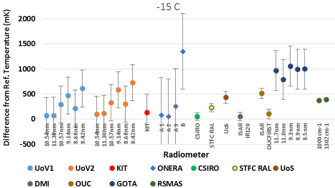
Figure 4: Plot of the mean of the differences of the radiometer readings from the temperature of the NPL reference blackbody, maintained at a nominal temperature of -15 °C.
