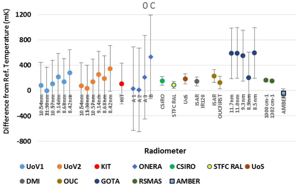
Figure 5: Plot of the mean of the differences of the radiometer readings from the temperature of the NPL reference blackbody, maintained at a nominal temperature of 0 °C.
