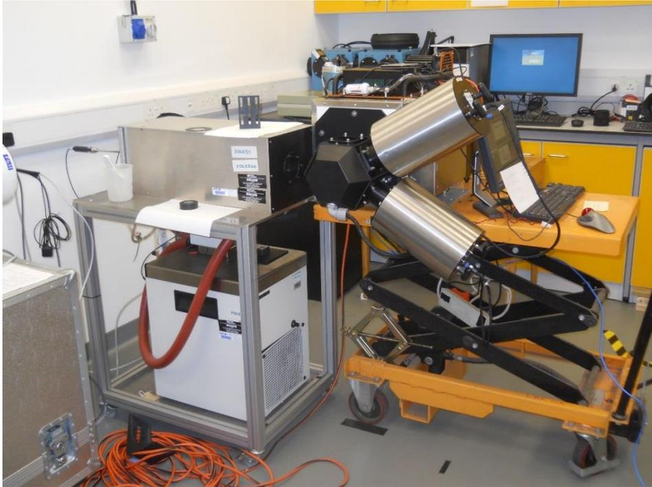
**Figure 1:** The RASMAS M-AERI radiometer viewing the ammonia heat-pipe blackbody during the 2016 radiometer comparison.
