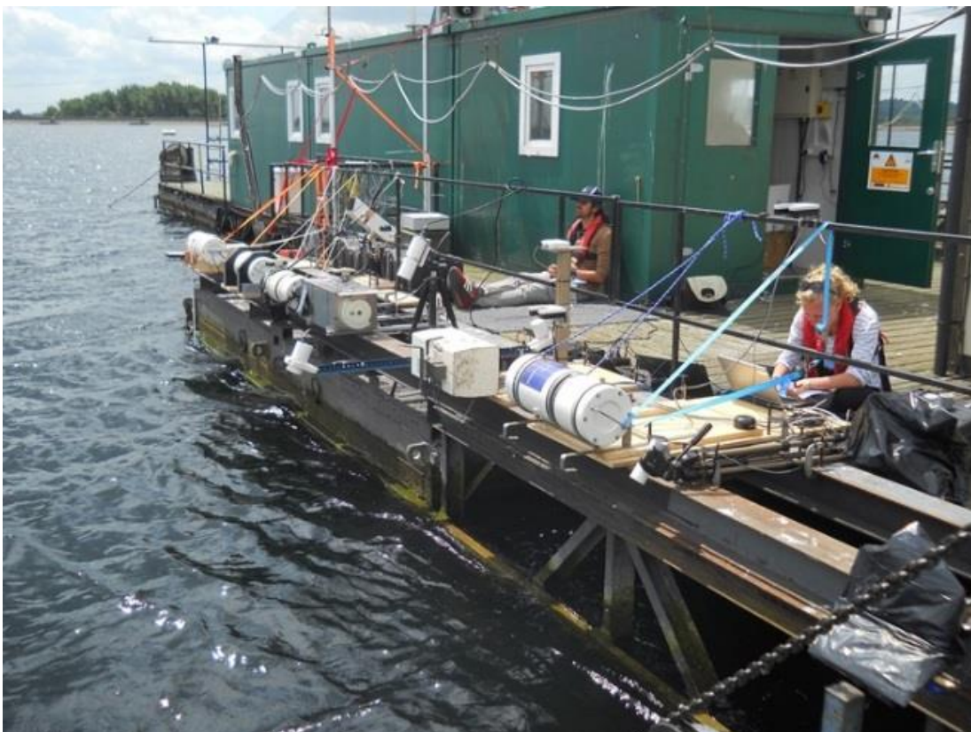
Figure 6: The participating radiometers mounted on the platform at Wraysbury reservoir and making measurements of the WST during the 2016 WST comparison.
