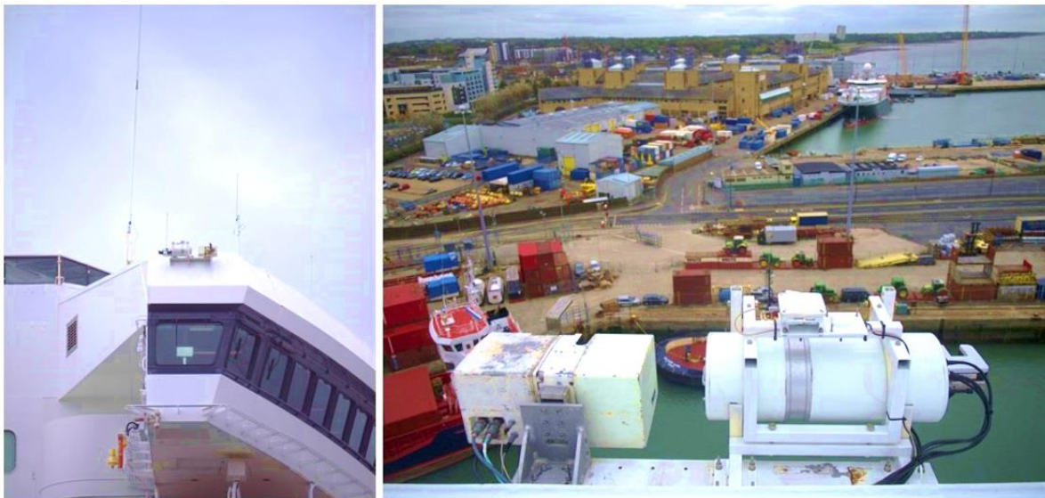
Figure 13: Left - SISTeR and ISAR side by side on the port side of the QM2 bridge roof. Right - SISTeR (left) and ISAR (right) mounted side by side.
