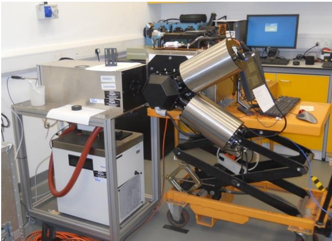
Figure 3: The radiometer lab comparison involved sequentially moving the participating radiometers in front of the NPL reference ammonia heat-pipe blackbody and measuring its radiance temperature. The photo above shows the RSMAS radiometer viewing/measuring radiance temperature of the reference blackbody.
